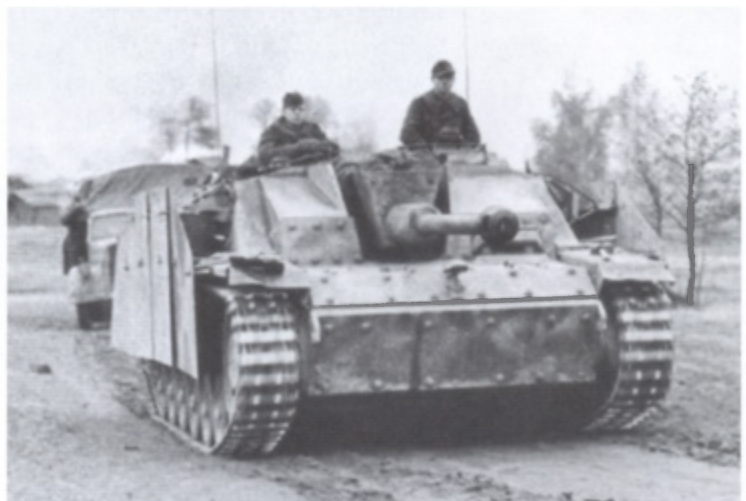
A Sturmgeschütz III Ausf. G on the Eastern Front. The first variant of the StuG III armed with the 75mm L/43 or L/48 long-barrelled gun was produced from March 1942, but the new version of this assault gun only entered mass production at the end of the year with more than 7,700 built up to March 1945. (Private collection)
